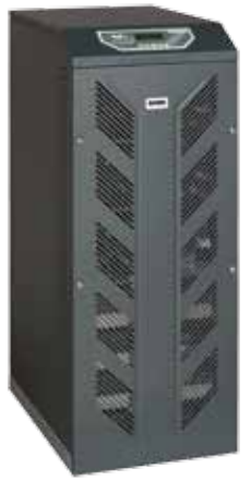
B8000FXS Series, 3/3 and 3/1 phase UPS, 10 to 100 kVA. On-line double conversion, transformer-free topology, full IGBT technology, parallelability up to 600 kVA.
