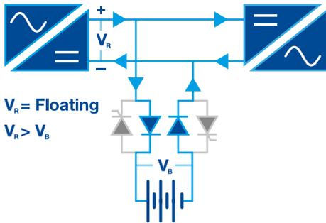
Battery is charged controlling the dynamic battery switch diodes on an intermittent basis, as per battery manufacturers recommendations, or after a discharge has occurred.
