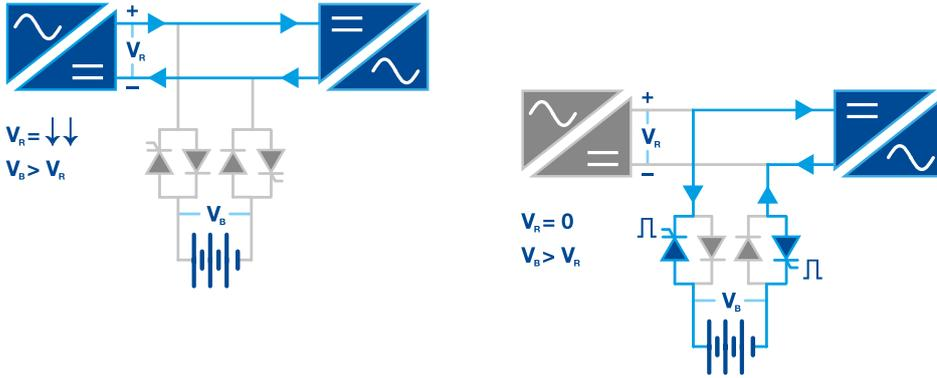
When battery is charged and mains are stable, it is protected from the DC-link ripple by a Green Conversion solid state dynamic battery switch, acting as a digital filter eliminating the chief cause of battery ageing. Green Conversion inverter control enhances system efficiency by reducing IGBTs commutation losses. During mains outages Green Conversion controls the dynamic battery switch SCRs and the battery feeds the inverter.
