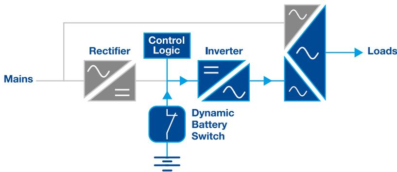
Ultra High Efficiency on-line mode: the inverter feeds power to critical loads whenever mains quality is outside tolerance limits.
