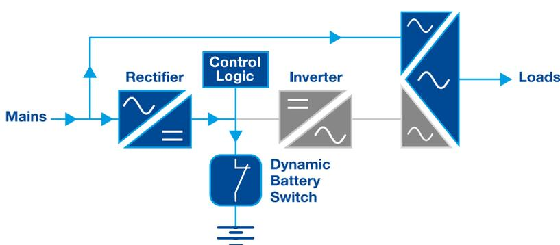
Ultra High Efficiency interactive mode if input mains stability and reliability is outside preset limits, this mode of operation is activated. Loads are fed by the mains and the inverter is turned on and off by the control logic to stabilize UPS output and the rectifier keeps full battery capacity. That's what we call Very High Efficiency (VHE) mode. Efficiency is 97%, due to the transient inverter and rectifier contribution to overall losses.
